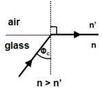
The critical angle can be defined as: the angle of incidence in the higher density medium corresponding to an angle of refraction of 90° in the lower density medium.
