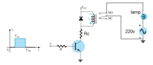
We use Vcc=5VFor the transistor to operate as a switch, this constraint should be followed:
