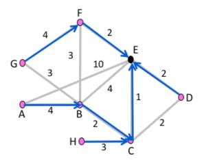
**b)** The source tree for **A**, using Dijkstra's algorithm.
