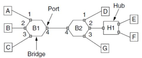
(a) *B1* will forward this packet on ports 2, 3, and 4. *B2* will forward it on 1, 2 and 3.
